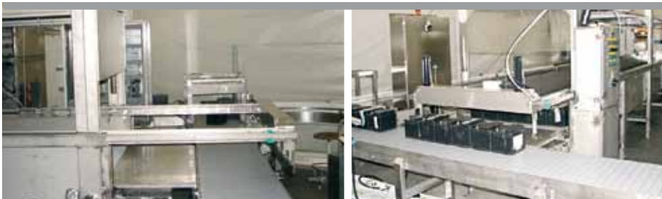
built-in devices for the automatic loading & unloading operations
