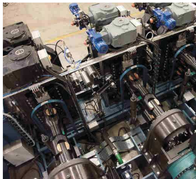
Top view of the powerful driving and roll pressure motors that are required to produce the necessary reductions and tight tolerances of the wide cast strip.
